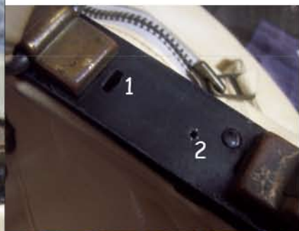
an original hole (1) and an additional one on the frame are used to install shoulder strap holders
